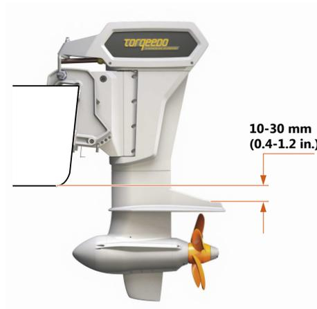
Fig. 45: Installation position
