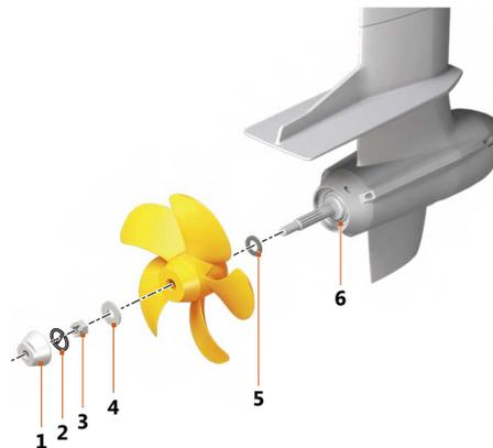
Fig. 71: Propeller attachment
