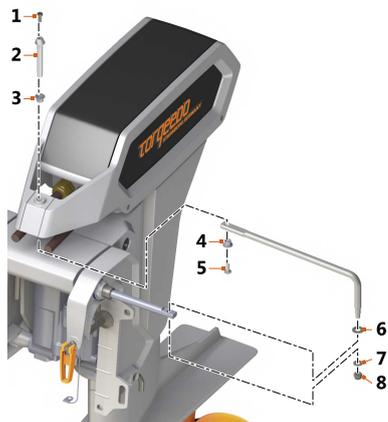
Fig. 48: Components of remote steering
