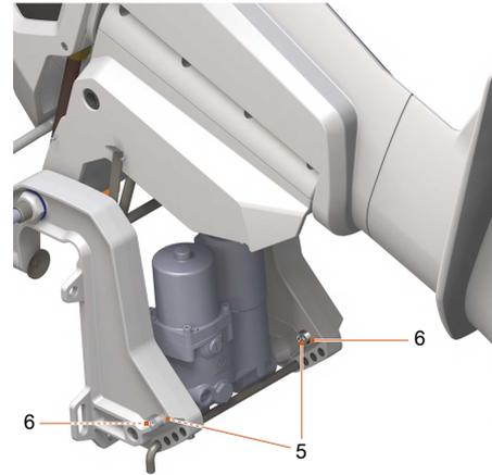
Fig. 74: Galvanic anodes for transom bracket
