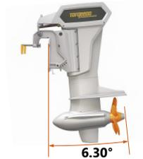
Fig. 70: Motor is tilted fully downwards
