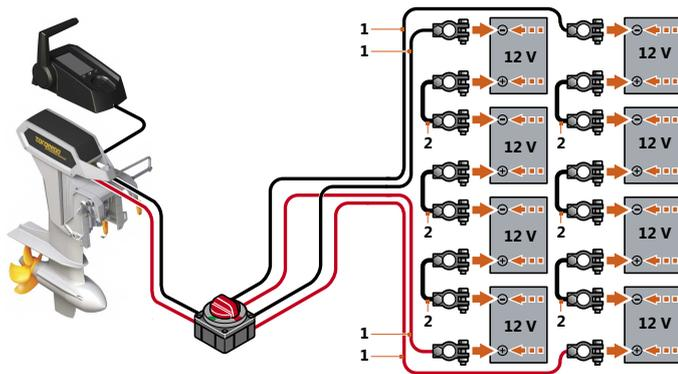
Fig. 54: Wiring diagram for lead batteries
