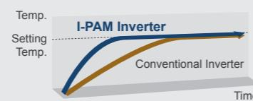
In addition, the voltage is raised at the start of operation and fast comfort is attainable by more powerful operation.
