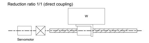
Screw pitch 10 [mm], transfer mass 20 [kg], thrust 0 [kg] (absent)
