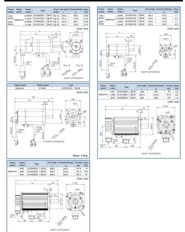
\* See page 8-27 for the shaft extension specification of the motor with a key.
