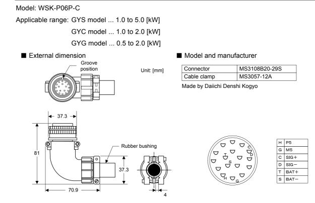
• The connector model is different from that of the option cable.
