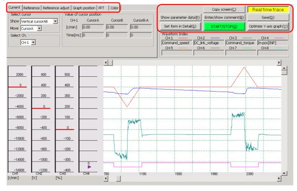
You can show the interval between two points, overlap waveforms, perform FFT analysis, copy the screen, show parameter data of the acquired waveform, save the waveform (in a CSV file), or do other things.
