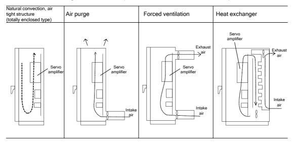
(3) To install two or more servo amplifiers in the same control panel, the following shall be taken into consideration.
