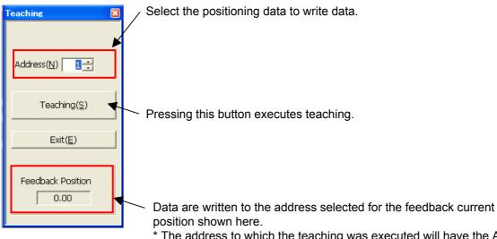
\* The address to which the teaching was executed will have the ABS type command method. Other setting will not be changed.
