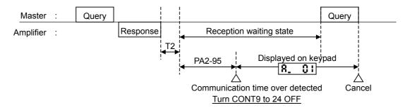
If PA2\_95 is set to 0.00 [sec], communication time over is not detected. Use this setting as needed, for example, if the system communicates periodically and you wish to detect discontinuation of the communications.
