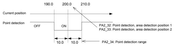
(2) PA2\_31 (point detection, area detection) = 1: area OFF → ON
