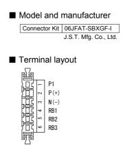
Motor power cable connector kit (amplifier side)
