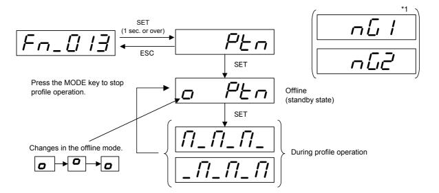
\*1) If NG indication is shown, remove the cause of the fault and press the [MODE/ESC] key to restart the offline state.
