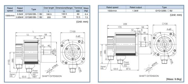
\* See page 8-27 for the shaft extension specification of the motor with a key.
