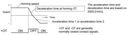
• If 1 (stop) is selected with parameter PA2\_24 (selection of operation at OT during homing), stoppage occurs according to parameter PA2\_60 (third torque limit). In this case, the homing motion is stopped upon detection of OT.
