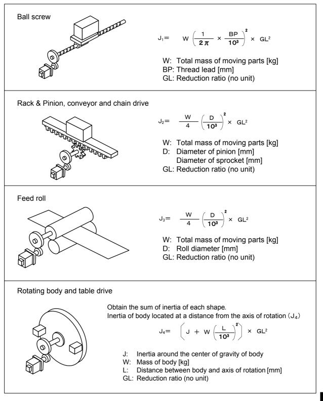
■ Calculation of load torque (TL)
