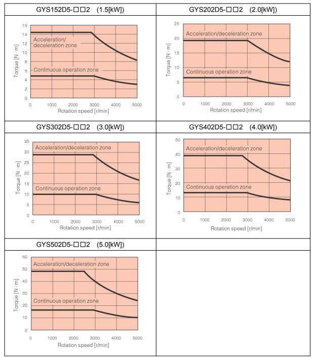
These characteristics indicate typical values of each servomotor combined with the corresponding RYT type servo amplifier. The rated torque indicates the value obtained when the servo amplifier is installed to the following aluminum heat sink.
