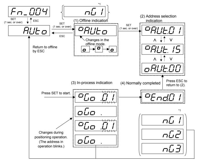
\*1 If NG indication is shown, remove the cause of the fault and press the [MODE/ESC] key to return to the offline state (2).
