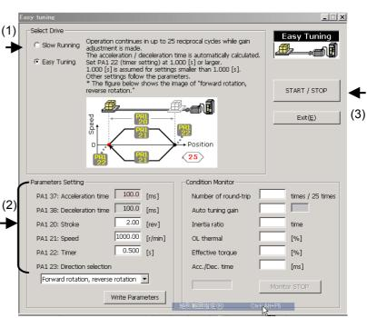
Hint Slow running is unnecessary for machines with a rotary driving system.
