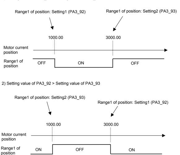
Note: If setting 1 of range 1 of position (PA3\_92) is the same as setting 2 of range 1 of position (PA2\_93), range 1 of position is always turned off. The same is true for range 2 of position.
