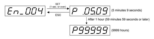
(5) Total time - control power supply The cumulative time of turning the control power (L1C and L2C) on is displayed. The displaying range is from 0 [h] to 9999 [h].
