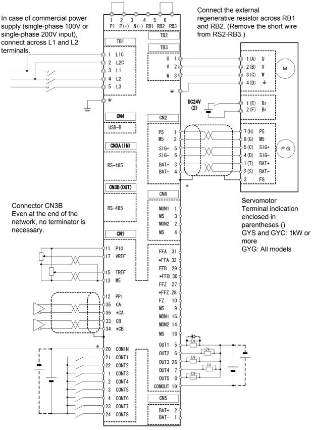
\* Connect the shielding wire to the connector shell on the servo amplifier side.
