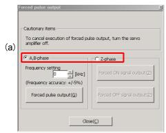
Select the pulse signal to be output, at (a).
