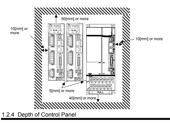
Reserve 80 [mm] or a wider space in front of the servo amplifier which is connected with sequence I/O cables and encoder cable.
