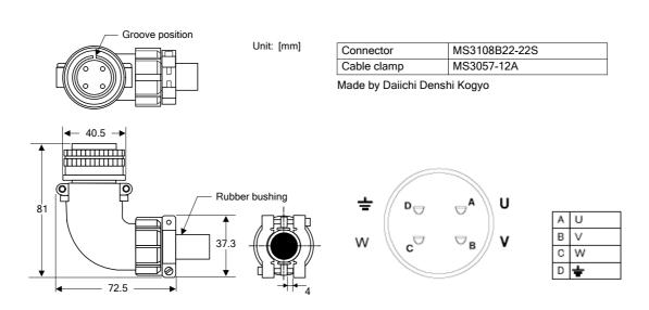
Connector kit for motor power wiring (motor side : with brake)
