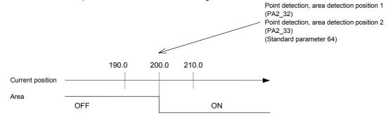
(3) Area  $ON \rightarrow OFF$  (If PA2\_31 (point detection, area detection) is 2)
