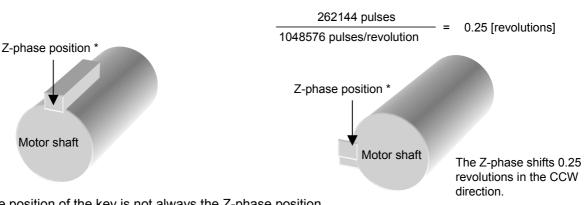
\* The position of the key is not always the Z-phase position.
