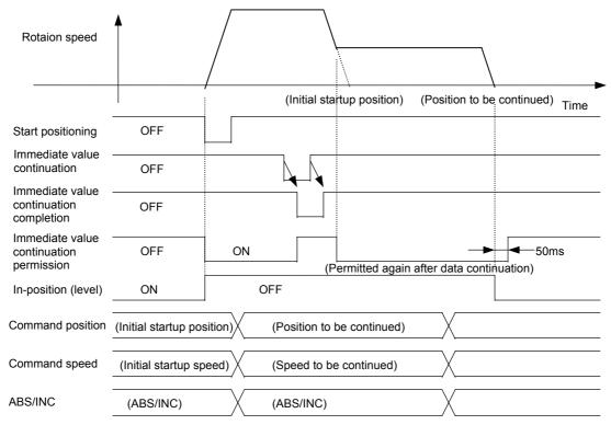
To allocate the immediate value continuation command to a sequence input terminal, enter the corresponding value ("22") in the input terminal function setting parameter. Relevant signal reference values include following.
