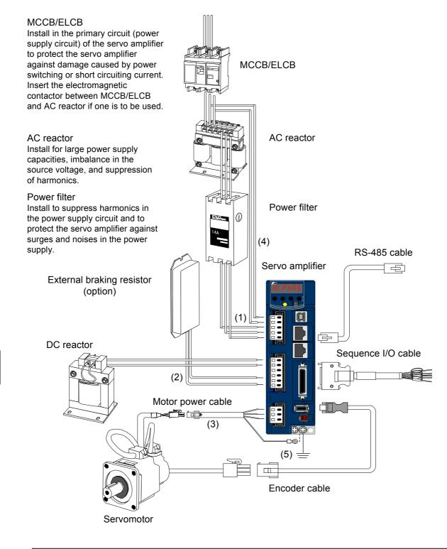
Wiring connectors do not come with the servo amplifier or servomotor. Prepare the necessary option cable or connector kit.
