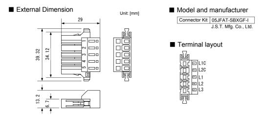
Intermediate circuit wiring connector kit (amplifier side) \* Provided with amplifier.
