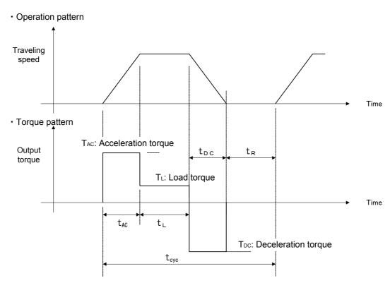
(6) Calculating the effective torque (Trms)Calculate the effective torque of each cycle of the operation pattern.
