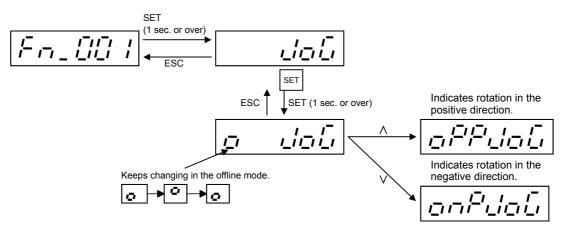
After checking shaft rotation in the test operation mode, press the [MODE/ESC] key to return until [Fn\_001] is displayed again.
