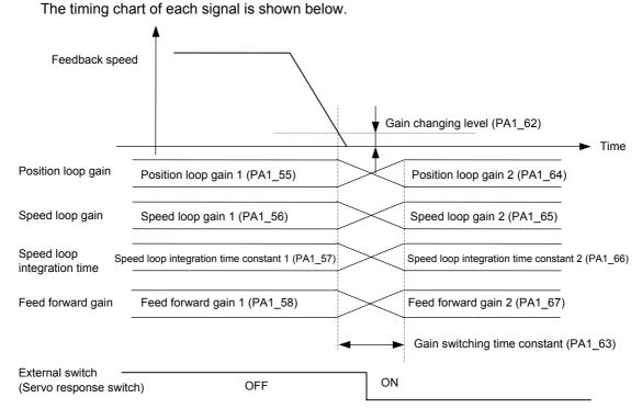
If external switch is selected as a gain changing factor, changeover to the second gain occurs during OFF-to-ON transition as shown above. In this case, you can turn on or off at an arbitrary timing without relations to the motor motion.
