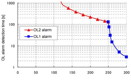
(1) In case of operation at rated rotation speed (1500/2000 [r/min])
