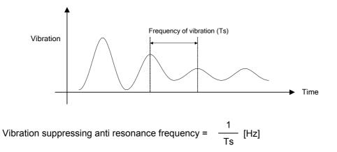
2) Starting at 300.0 [Hz] (maximum setting), decrease the reference values of parameters PA1\_78, \_80, \_82 and \_84 gradually while visually checking vibration, to find the best value.
