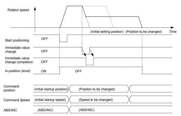
The command position and command speed change at the activating edge of the immediate value change command. They can be changed at an arbitrary timing while the in-position signal remains inactive.
