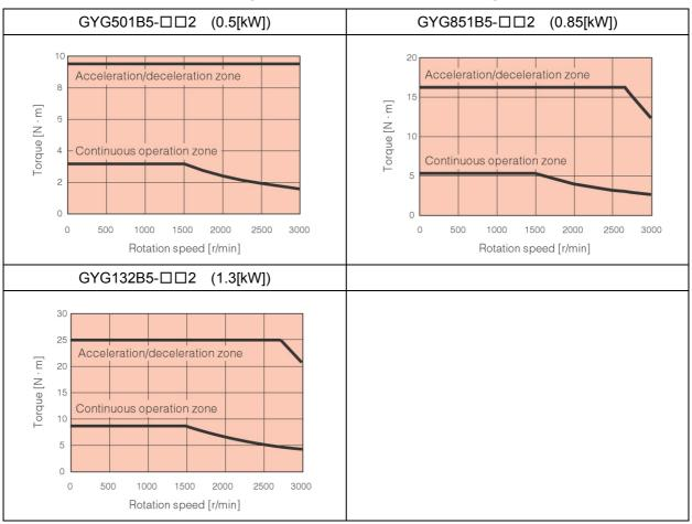
■ Torque characteristics drawing (at 3-phase 200 [V] source voltage)
