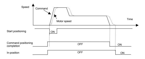
If the command positioning completion signal is allocated to an output signal, the condition for the next start signal is activation of the command positioning completion signal. Refer to the timing chart below.
