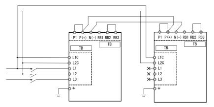
When performing PN junction as shown in the figure above, it is recommended to use a marketed connecter: CL-1814T (made by JST) by preparing it separately. It is because two wires cannot be connected to the connector (WSK-S05P-E, WSKR06P-E) of the servo amplifier of frame 4 or less. (The following figure is a connection example of control power supply part.)
