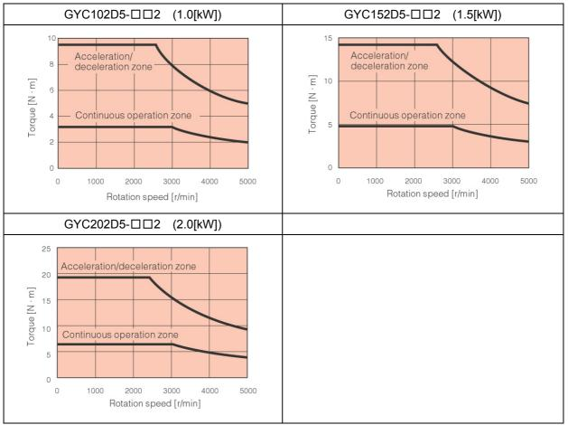
These characteristics indicate typical values of each servomotor combined with the corresponding RYT type servo amplifier.
