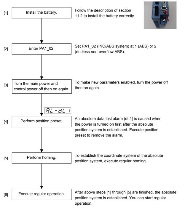
• If the encoder cable is disconnected due to transportation or device changes, repeat the procedure from step [4].
