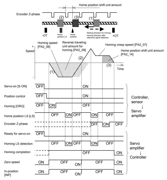
• At the direction of rotation switch rotation direction selection point with zero speed, zero speed and in-position [INP] are momentarily turned on. The signal change may fail to be sensed according to some scanning periods of the host controller.
