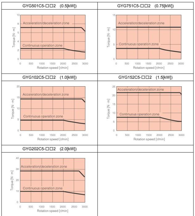
Torque characteristics drawing (at 3-phase 200 [V] source voltage)
