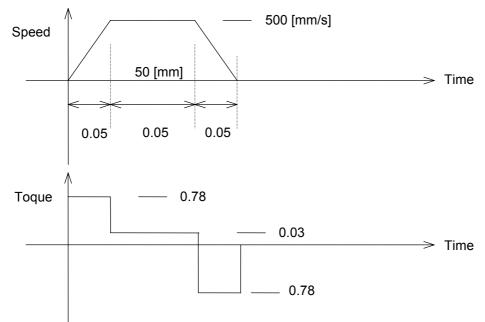
This profile is based on calculation selection. The operation cycle time supposes 0.5 sec.
