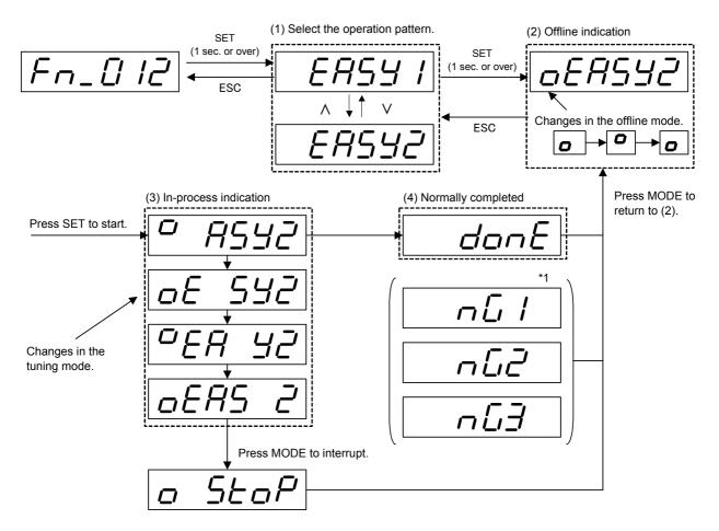
\*1) If NG indication is shown, remove the cause of the fault and press the [MODE/ESC] key to return to the offline state (2).
