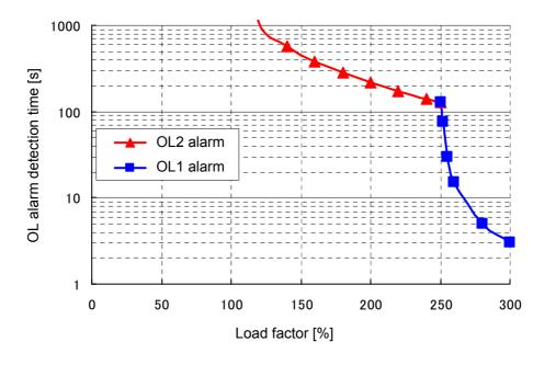
(2) In case of operation at maximum rotation speed (6000 [r/min])
