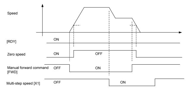
Use parameter PA3\_35 to specify the zero clamp level in relation to the [VREF] input.
