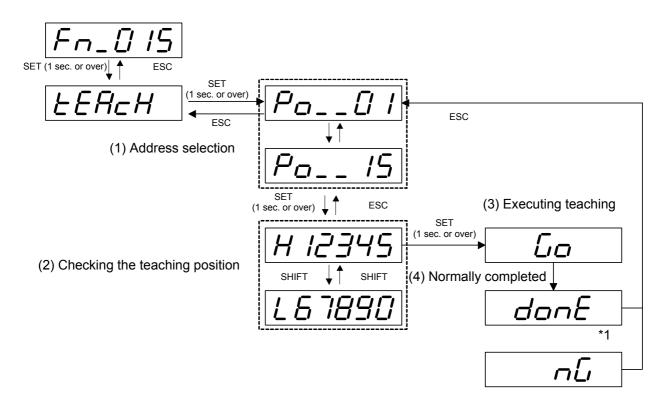
\*1 If NG indication is shown, remove the cause of the fault and press the [MODE/ESC] key to return to the address selection (2).
