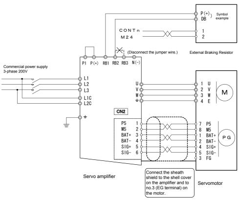
To use an external braking resistor, wiring and parameter setting are necessary.
