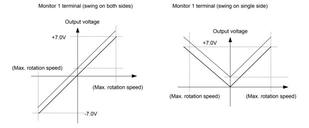
Specify the negative sign for the monitor 1/2 scale to reverse the polarity of the output voltage.
