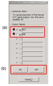
Select the OUT signal output at (a) and select ON or OFF at (b).
