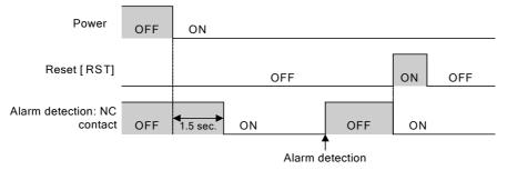
The contact remains turned off for about 1.5 seconds after the power is turned on.
