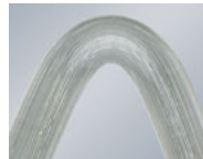
A 217-core fiber is hardly affected by excessive bending.
