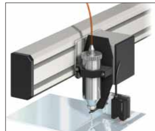
Controlling the nozzle height of a dispenser
