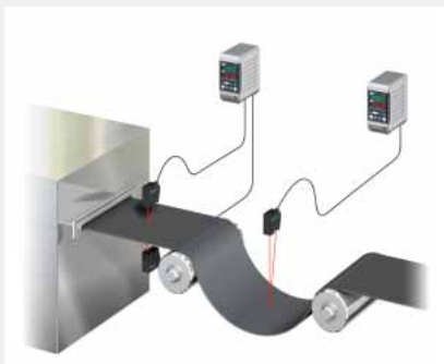
Thickness measurement/loop control of a rubber sheet
