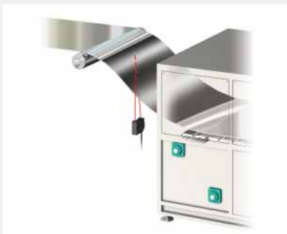
Monitoring free loop control
