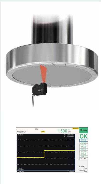
Flatness of a wafer polishing machine
