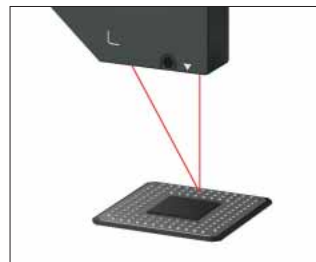
Measuring the shape of BGA
