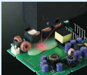
Height measurement of PCB resin
