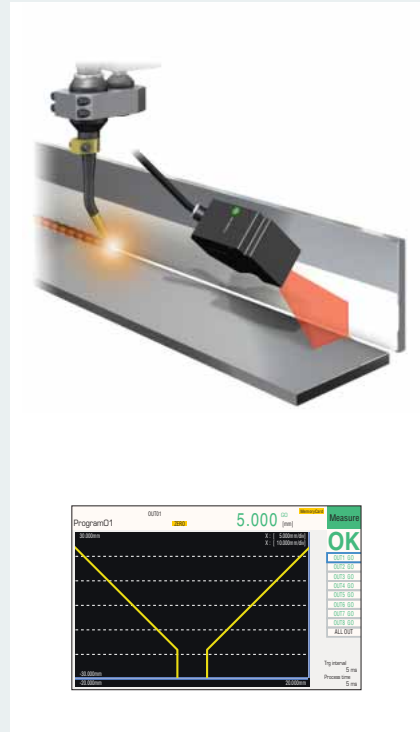
Position feedback in an automated welding operation
