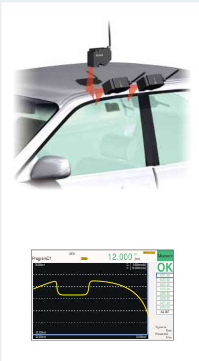
Checking the assembly accuracy of an auto body
