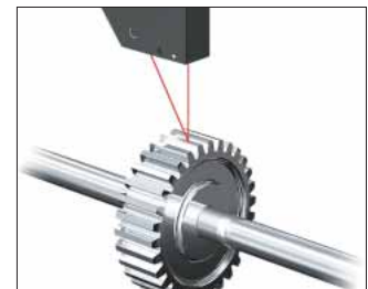
Measuring the surface profile of a gear
