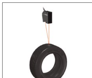
Measuring the shape of a tire
