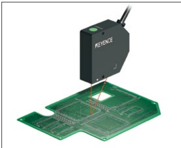
Measuring the warpage of a PCB
