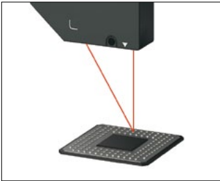
Measuring the shape of BGA
