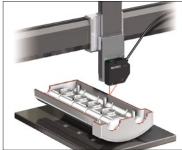
Measuring the height of liquid sealant
