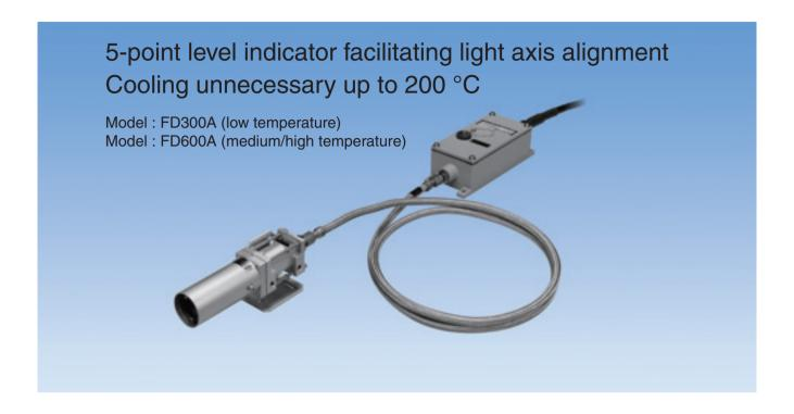
The optical head and amplifier are connected with a fiber optic cable and the infrared ray captured with the optical head is transmitted through highly transmissive glass fiber into an amplifier installed at a distant location. The infrared ray transmitted into the amplifier is optically converted in the light-sensitive element and amplified for control signal output (mini power relay, relay or Solid-state output).
