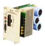
This single-axis, Direct PWM amplifier is designed to fit into a standard 3U UMAC rack. It is intended for driving AC induction, permanent magnet brushless, linear, and brushed DC motors. It has a current rating of 8.0 A Continuous/16.0 A Peak.
