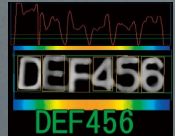
Height-extracted image (Free-form plane) + OCR
