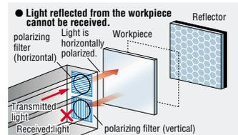
Light that has been horizontally polarized at the transmitter cannot pass through the vertically oriented polarizing filter even if it is reflected from the workpiece before reaching the reflector.
