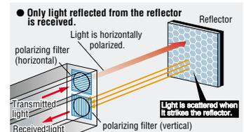
Light is scattered as it strikes the reflector, allowing it to be received regardless of the orientation of the polarizing filter.
