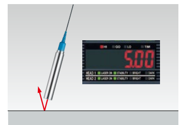
When the sensor is installed at an angle to the target: A sufficient amount of reflected light is not returned to the sensor.
