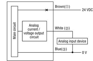
Pin layout when the M12 connector (4-pin) cable is used
