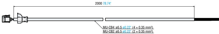
Sensor-to-controller cable (4-pin M12 connector type)
