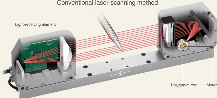
The laser beam is projected onto a rotating polygon mirror, the reflected light scans the measurement range, then reaches the receiving element. To improve speed and accuracy the motor would need to rotate at a faster rate at the cost of durability and reliability.
