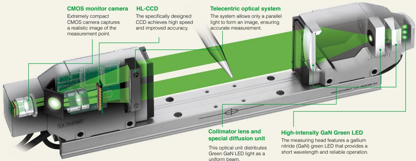
The LS-7000 Series features an optical system with a green LED a telecentric lens a HL-CCD. Helping achieve double speed and accuracy compared to conventional micrometers. The motor-less structure and longer-life light source ensure excellent durability that retains reliable operation for a long time.
