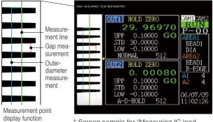
\* Screen sample for "Measuring IC lead pitch" on page 5.
