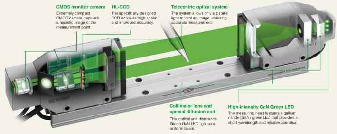
The LS-7000 Series features an optical system with a green LED a telecentric lens a HL-CCD. Helping achieve double speed and accuracy compared to conventional micrometers. The motor-less structure and longer-life light source ensure excellent durability that retains reliable operation for a long time.
