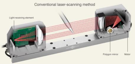
The laser beam is projected onto a rotating polygon mirror, the reflected light scans the measurement range, then reaches the receiving element. To improve speed and accuracy the motor would need to rotate at a faster rate at the cost of durability and reliability.
