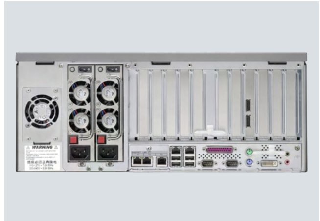
Rear of SIMATIC IPC847C with redundant power supply (optional)
