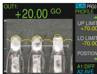
Soldered area of leads
