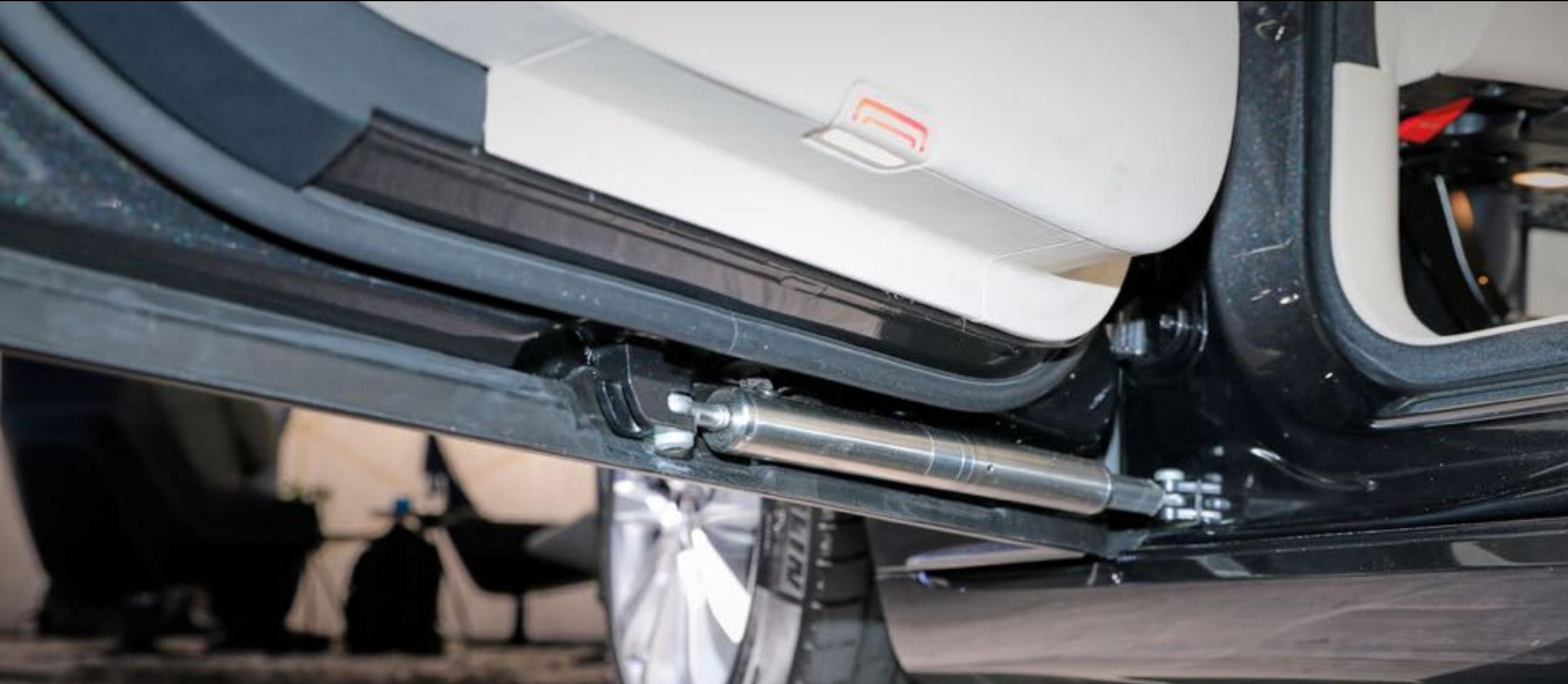
An actuator helps to open and close the doors and holds them in position when necessary. The doors can be opened with one hand when the car is on an incline - and the bodyguard who opens the door still has one hand free in the event of a defense.
