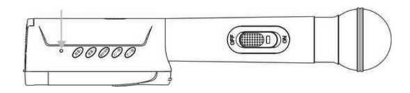
The indicator light is green when charging. The indicator is off when fully charged.
