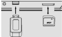
2. Following the illustration below, insert a USB device face up into the USB port, making sure it is fully inserted. Alternatively, insert a memory card in the direction of the arrow (as shown on the label next to the memory card slot), making sure to insert it straight without bending.
