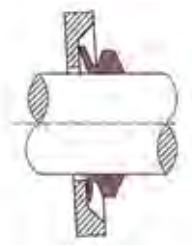
Improved lip design to compensate for shaft misalignments
