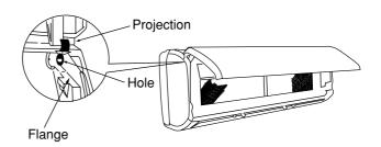
Move the projections of the left and right arms into the Flanges in the unit and securely insert them into the holes.
