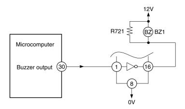
Fig. 3-1 Buzzer Circuit
