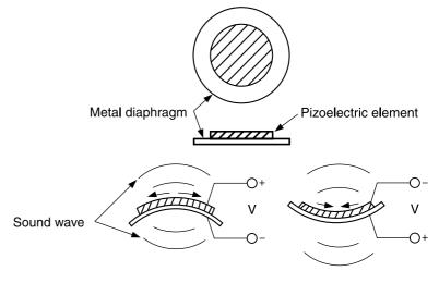
Fig. 3-2 Buzzer Operation
