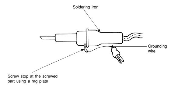
Fig. 4. Grounding a soldering iron
