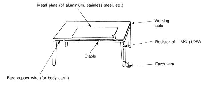
Fig. 3. Grounding of the working table
