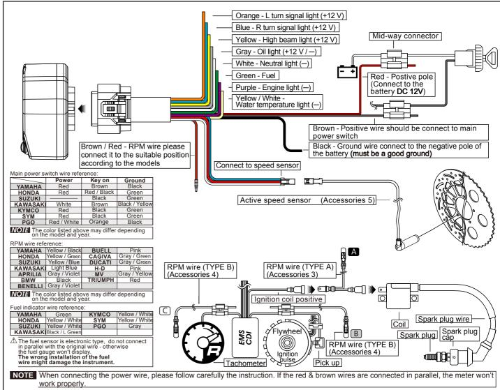
NOTE Motor oil indicator can be set up, install as two stroke motor oil indicator, or other positive(+12V) or negative actions' indicator.
