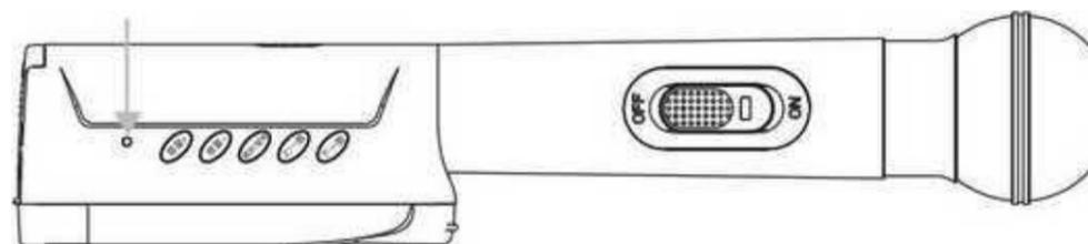
**The indicator light is green when charging. The indicator is off when fully charged.**
