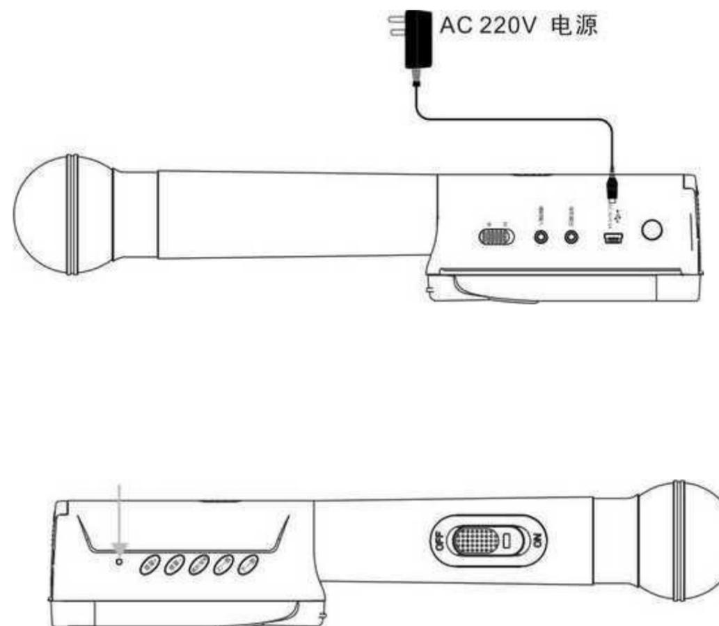
**The indicator light is green when charging. The indicator is off when fully charged.**
