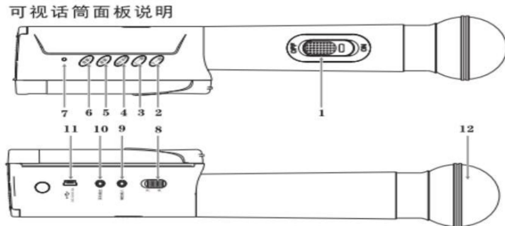
1. Switch for Visual Microphone: Turn the ON position to turn on the viewable microphone, turn it to the OFF position to turn off the viewable microphone, and dial to the middle position to be muted.
