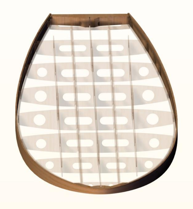
Attach 2 layers of hybrid rails
