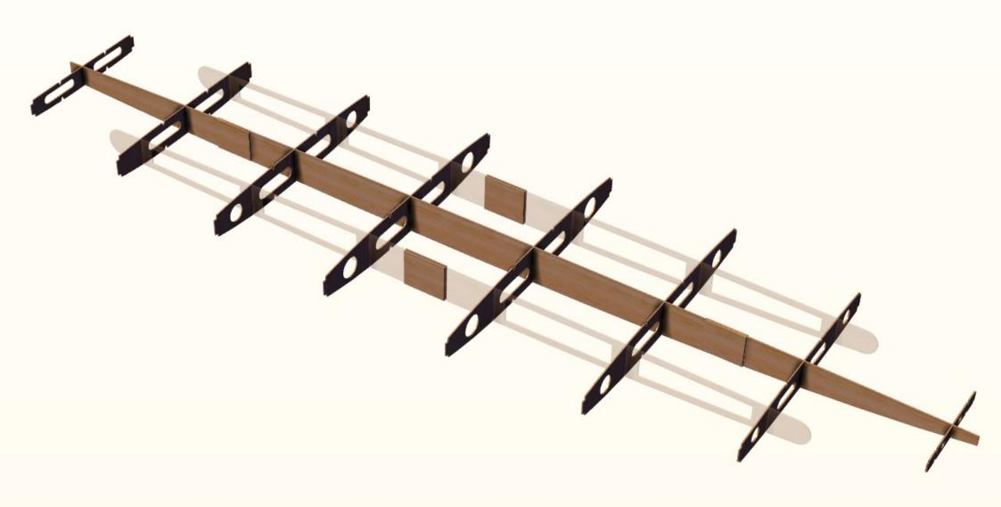
Connect Side Spline supporting block
