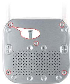
1) Unscrew the four fixed screws, remove the upper cover.
