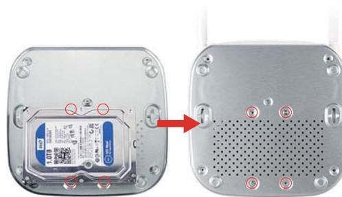
2) Fix the HDD on the bottom panel with screws.
