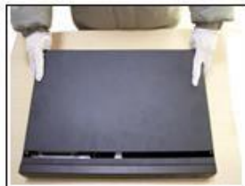
② disassemble the cover
