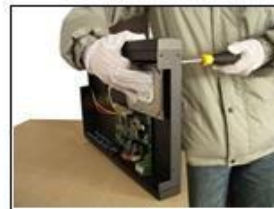
③ fix the screw of hard disk
