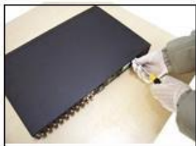
① disassemble the screw
