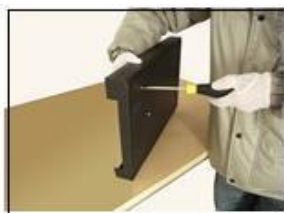
④ fix the screw of hard disk
