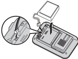
4 Attach and insert the replacement battery.
