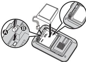
5 Insert the tabs (1) into the slots, and then close the battery cover (2).
