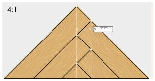
Measure the distance between the two straight lines, starting from the corners of the rods.
