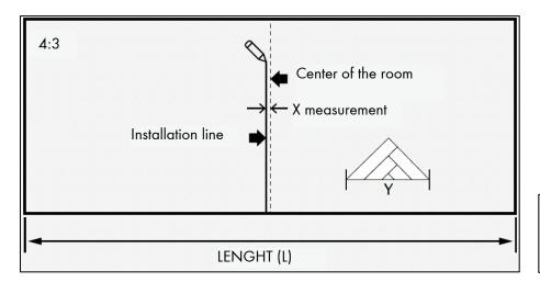
Drawing the installation line - Start from the center of the room. Parallel offset the line using the X measurement as the distance. Calculate the number of starting triangles needed using the formula below. Round to the next full number.
