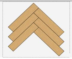
Install the rods precisely and in the order indicated by the numbers on the rods. Carefully check the joints between the rods, after each rod that is added. No protruding edge should be felt!
