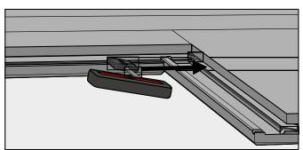
Insert the 5G dismantling pin into the hole of the guiding block. Insert the guiding block into the groove of the rod. Attention! The "UP" sign should be facing upwards.
