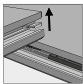
Push forward the 5G dismantling pin. The 5G dismantling pin pushes back the flexible tongue and releases the rod for dismantling. Now it is easy to lift the rod by its long side.
