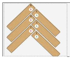
Take B rods and A rods and position them as shown above. The number of rods varies depending on the width of the rods used.
