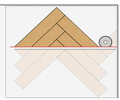
Cut the triangle according to the indicated red line. Depending on the type of saw, it may be useful to dismantle the triangle before sawing. The excess (below the line) is kept for the last line installation.
