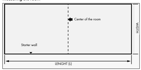
Define the wall from where you intend to start the installation. Mark the center of the room.
