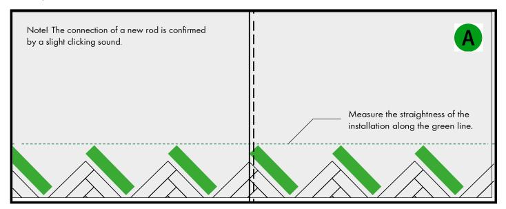
Now install the B rods and cut the edge rods to fit again with the required distance to the wall.
