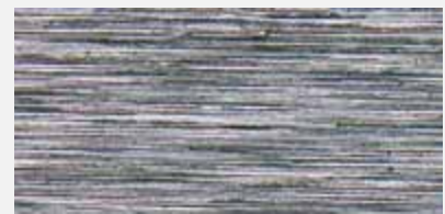
Abrasive belt 40 grit short distinctive line pattern, rough surface, high contrast finish
