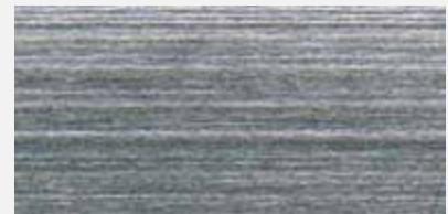
Abrasive mop wheel 40 grit long continuous line pattern, minimum depression, smooth finish
