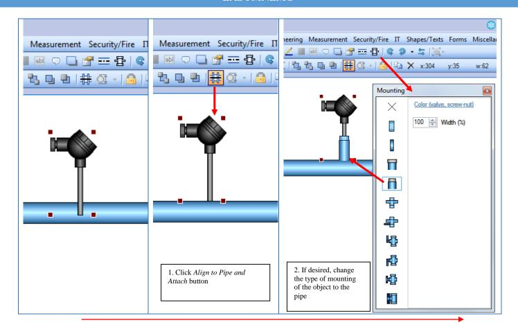
In addition, to visualize the installation there are special "mounting" elements. They are located in the *Measurement* section.
