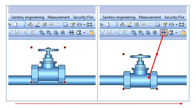
8. Some objects (for example, a pressure gauge or temperature sensor) can be tied to the border (surface) of the pipe. Click the button ##. To change the type of the mounting click the button ## (or click *Mounting* on context menu). Set your desired mounting in the *Mounting* dialog box.
