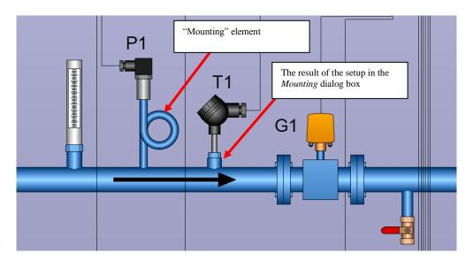
9. To set the object size by pipe diameter, click the button  $\square$  (or click  $Align > Set Object Size by Pipe Diameter on context menu). You can also press the button <math>\neg$  (located to the right of the button  $\square$ ) to set object size by pipe diameter with the multiplication factor.
