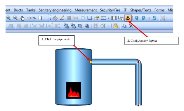
5. To change the diameter of the pipe, diameter, and color of individual segments of pipe and the type and size of pipe nodes click the button (or click *Nodes and Diameter* on context menu). Set your desired pipe diameter, segment diameter, node diameter, insulation, flanges and gaskets in the pop-up dialogue box.
