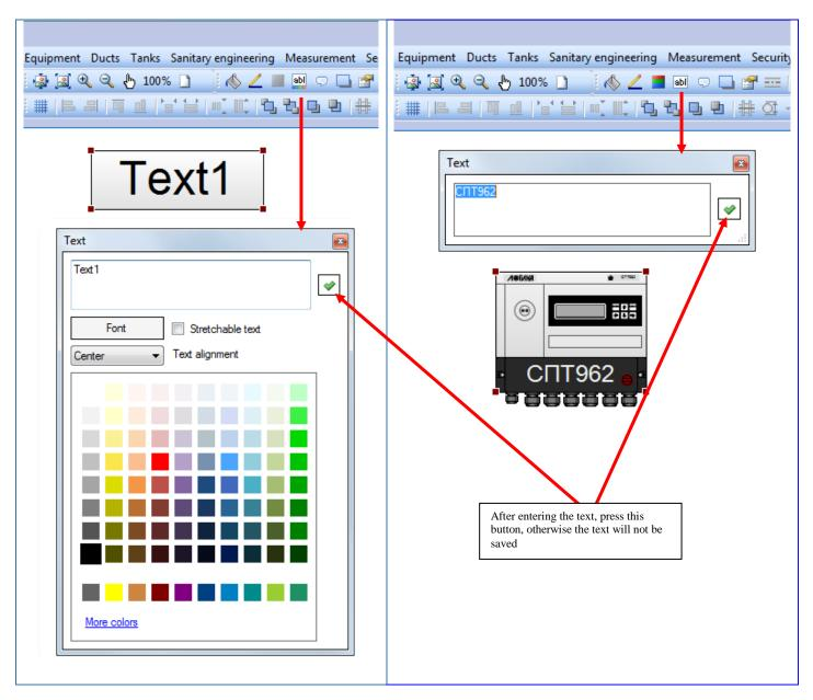
After entering the text, be sure to click on the button , otherwise the text will not be saved. If the *Stretchable text* check box is selected, the font size does not matter, the text size will depend on the size of the object.
