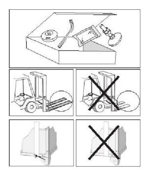
When lifting with forklift trucks or pallet jacks, ensure that the forks go under the entire length of the box, otherwise the underside of the box may be damaged. When using a crane, straps must be secured to legs or any pallets; it is important that the straps do not slip during lifting.
