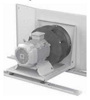
Dust can accumulate on the fan impeller which can cause imbalance and vibrations. The fan impeller must therefore be checked once a year and cleaned, if necessary. Anti-vibration mounts and flexible connections should be checked at the same time. If the anti-vibration mounts are damaged in any way they must be replaced.
