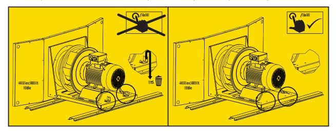
After disposal of the transport brackets the yellow label on the outside of the fan inspection door has no function and should be removed.
