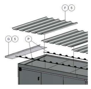
The trapezoidal roof plates are mounted with the self-drilling, painted screws supplied with sealing washer.
