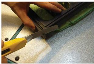
Push the filters carefully in the U-profile to be sure that there are no leakages between the filters Check that the vertical side of the last filter in the U-profile is fully even with the end of the U-profile. If the end of the last filter is not fully even with the end of the U-proflle an additional self-adhesive profile must be added to avoid any gap between the rubber profile on the inspection door and the last filter.
