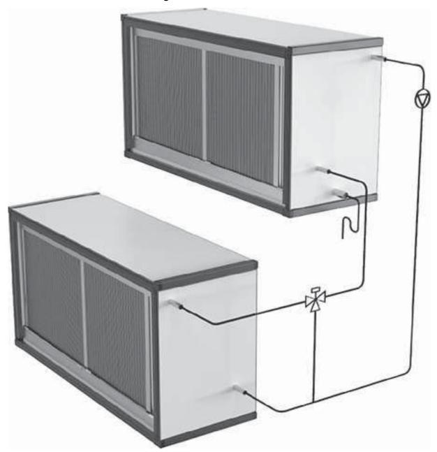
A heat recovery system of this type consists of a heating coil in the supply air- flow and a cooling coil in the exhaust air- flow. After an extended running period (normally a few years) dust particles can accumulate on the surface of the coils. This can reduce the efficiency of the coils. Cleaning must be carried out with the utmost care to ensure that the coil fins are not damaged.
