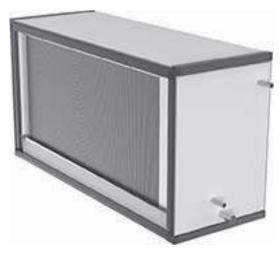
Once a year clean the drip tray beneath the cooling coil, as well as the drain and the water trap. Take care that there is sufficient water in the water trap. If a droplet eliminator has been fitted to the cooling coil, this must be checked once a year and cleaned if necessary.
