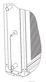
Coil seen from above. The sensor measures the water temperature of the water inside one of the small pipes for return water in the coil. The sensor reduces the area in this pipe and hereby also the flow of warm water in this pipe. The temperature in this pipe is reduced more than the temperature in all other pipes by the airflow through the battery. Because the lowest temperature in the battery probably is measured here, this system creates early and safe warning of frost.
