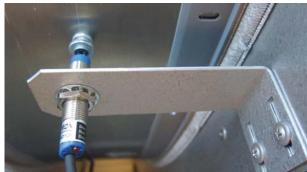
Mount the illustrated screw on the rotor for activation of signal from the sensor.
