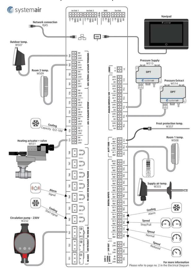
Terminals at the Access control board. The connected components is an example, and not unique for any order.
