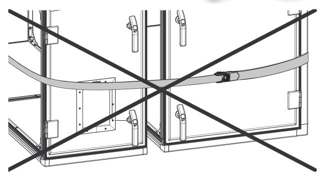
Note! Never — place the strap on the vertical profile when a section is pulled along the base frame or on the floor.
