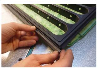
Remove excess of the strip. The end of the strip must be fully even with the horizontal side of the filter frame.
