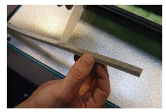
Place the self-adhesive strip on  $\ensuremath{\text{one}}$  vertical side of the filter fame
