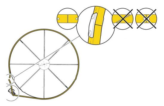
Check the drive belt annually. Replace if necessary. Reuse both brackets. If new screws are needed do not hesitate to make the screws even with the surface of the inner bracket.
