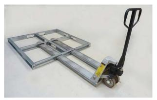
Do not activate the wheels of forklift on the horizontal profile of a middle profile. Activation of the wheels on the horizontal profile might bend the profile.
