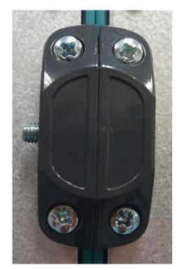
The grey guiding and connection blocks might be installed inside the units on the vertical profiles. Press the sections hard together so that the rubber profiles are so flat that the iron frames of the two sections are joined. Strap with tensioner is suitable for pressing the sections hard together. Note! Do not place the strap on the vertical profiles. To avoid any load and stress on the profiles the strap must be carefully placed on the bottom profiles of the unit.
