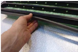
Check that the end of the strip is fully even with the horizontal side of the filter frame.
