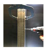
Bracket inside a section. A similar bracket is installed in the next section. This is the bracket in the Geniox sizes 10 and 18
