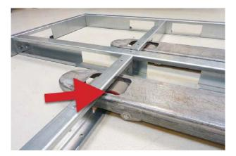
The forks of the forklift must be longer than the width or length of the section/unit to achieve safe transport of the section/unit.
