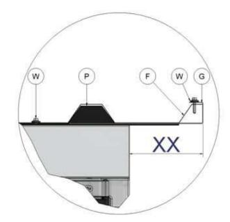
The unit is delivered with 2 similar overhang profiles - G1 and G5 - one for each end of the roof. Mount one of the 2 roof overhang profiles - G on a trapezoidal roof plate. Use the self drilling, painted screws with sealing washers - W - see the illustration.
