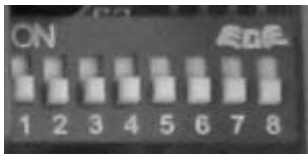
The 8 DIP switch levers
