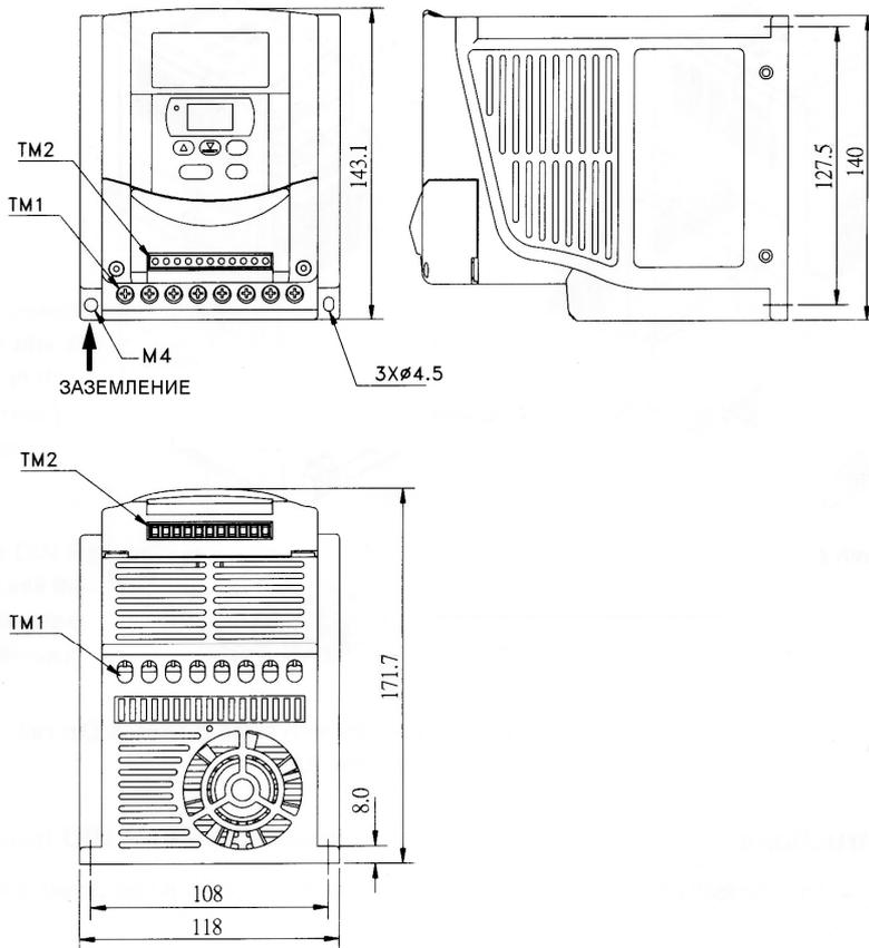
**Типоразмер 3: SP25L-IP65, SP5L-IP65, S1L-IP65**
