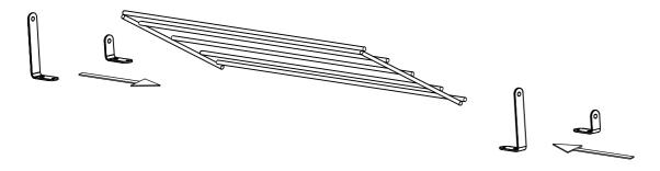
2- Fix long and small L-shaped part to cabinet doors with chipboard screw.
