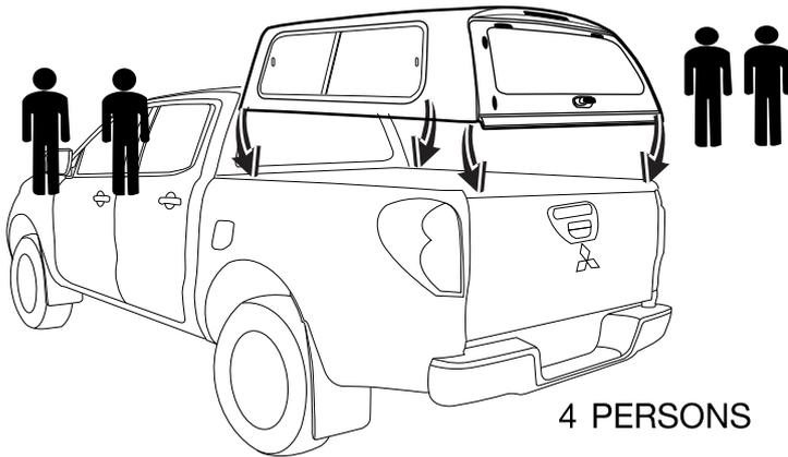
**4** Adjust alignment between front and rear and arrange left and right.
