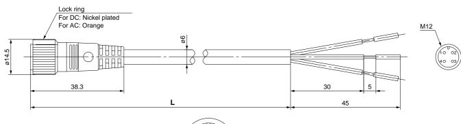
Socket pin connector pin assignment
