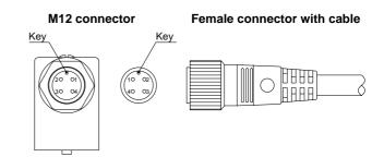
Note) For connecting a female connector with cable, adjust the connector key to the M12 connector key in the valve side since there is an orientation.
