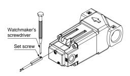
When tightening the auto switch mounting screw, use a watchmaker's screwdriver with a handle of approximately 5 to 6 mm in diameter. Furthermore, use a tightening torque of approximately 0.10 to 0.20  $N {\, \cdot \,} m.$
