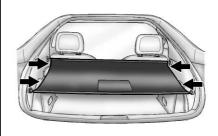
There is a cover for the rear cargo area. Use the four cargo cover loops to hook the cover to the side panels.
