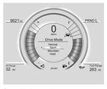
Sport Mode provides more responsive acceleration than Normal Mode, but can reduce efficiency. Use Normal Mode whenever possible.
