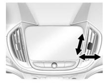
Use the louvers on the air vents to change the direction of the airflow, or to open and close off the airflow.
