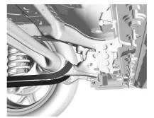
3. If the car is parked at an angle so that the front toe eye cannot be accessed, wrap a tow strap around both of the rear trailing arms and pull the vehicle onto a flat surface. Do not wrap the tow strap around the rear torque tube.
