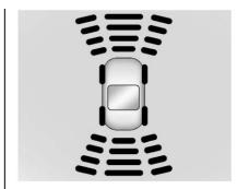
The instrument cluster may have a parking assist display with bars that show "distance to object" and object location information for RPA, and on some vehicles, FPA. As the object gets closer, more bars light up and the bars change color from yellow to amber to red.
