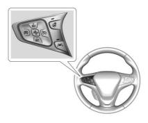
ৈ: Press to turn the cruise control system on and off. A white indicator comes on in the instrument cluster when cruise is turned on.
