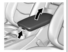
There is storage under the armrest. Press the button and lift to access.
