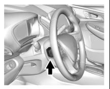
Regen on Demand allows increased deceleration by pressing and holding the steering wheel paddle. It works in D (Drive) and L (Low). The accelerator pedal must be fully released for it to work.
