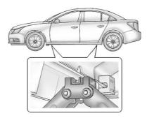
Position the jack lift head at the jack location nearest the flat tire. The location is indicated by a notch on the bottom edge of the body side. The jack must not be used in any other position.
