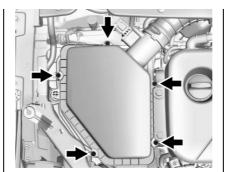
Remove the five screws and lift the air cleaner/filter cover from the air cleaner/filter housing assembly.
