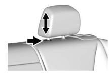
The height of the head restraint can be adjusted. Pull the head restraint up to raise it. Try to move the head restraint to make sure that it is locked in place. To lower the head restraint, press the button on the top of the seatback, and push the head restraint down. Try to move the head restraint after the button is released to make sure that it is locked in place.
