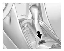
Pressing MODE will display the selectable drive modes in the Driver Information Center (DIC). See *Driver Selected Operating Modes* \$\dip 181\$ for information on mode operation.
