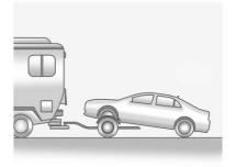
The vehicle can be towed from the front using a dolly. To tow the vehicle using a dolly:
