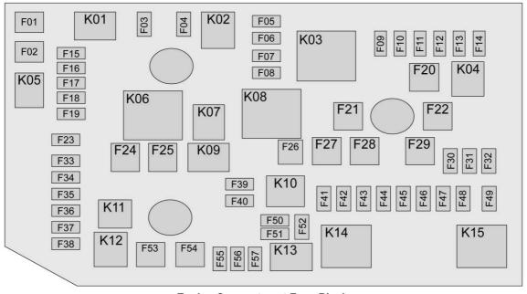
**Engine Compartment Fuse Block**
