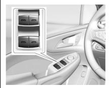
The window switches on the driver door control all windows. Each passenger door has a switch that controls only that window.
