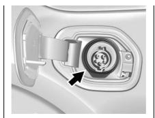
If equipped, the charge port bezel light acts as an additional CSI when the vehicle is plugged in and charging. It will flash along with the CSI on the instrument panel.
