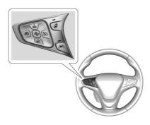
(iii): Press to turn the cruise control system on and off. A white indicator comes on in the instrument cluster when cruise is turned on.
