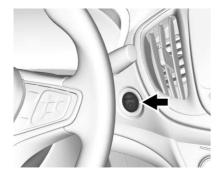
The vehicle has an electronic pushbutton start. The POWER  $\circlearrowleft$  light flashes when the driver door is open and the vehicle is not on. The flashing light will eventually time out. The light is on steady when in ON/
