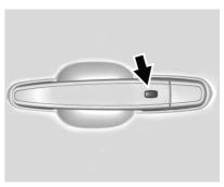
When the Remote Keyless Entry (RKE) transmitter is within 1 m (3 ft) of the driver door, the door can be locked and unlocked by pressing the door handle button. When unlocking from the driver door, the first press will unlock only that door; press again within five seconds to unlock all passenger doors. See Remote Keyless Entry (RKE) System Operation ⇒ 30.
