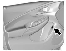
Press the fuel door button on the driver door for one second. A WAIT TO REFUEL message displays on the Driver Information Center.
