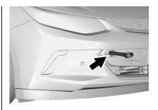
5. Screw the tow eye bolt into the bumper.
