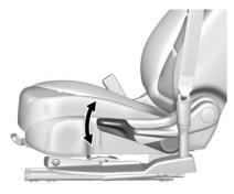
Move the lever up or down to raise or lower the seat.
