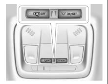
The dome lamp controls are in the overhead console.
