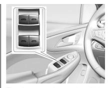
Press or pull the switch to open or close the window.
