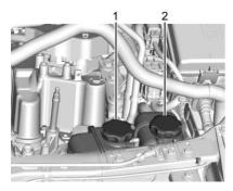
1. High Voltage Battery Coolant Reservoir
