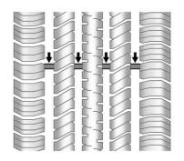
Treadwear indicators are one way to tell when it is time for new tires. Treadwear indicators appear when the tires have only 1.6 mm (1/16 in) or less of tread remaining. See *Tire Inspection* ⇒ 284 and *Tire Rotation* ⇒ 284.
