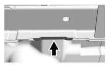
The hoist arm pad and jack stands must be placed on this recessed area of the flange.
