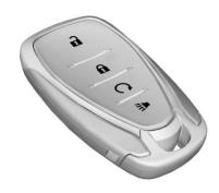
**a**: Press once to unlock the driver door or all doors depending on the vehicle personalization. Press a second time within five seconds to unlock all doors.
