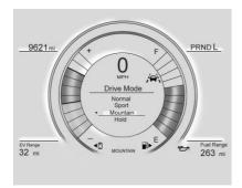
Mountain Mode should be selected at the beginning of a trip before climbing steep, uphill grades and when expecting to drive in very hilly or mountainous terrain. This mode maintains a reserve electrical charge of the high voltage battery to provide better grade climbing performance. While driving in Mountain Mode, the vehicle will have less responsive acceleration.
