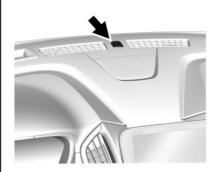
The vehicle has a Charging Status Indicator (CSI) at the center of the instrument panel near the windshield. When the vehicle is plugged in and the vehicle power is off, the CSI indicates the following:
