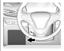
The instrument panel fuse block is on the left side of the instrument panel. To access the fuses, open the fuse panel door by pulling out.
