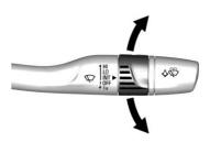
**INT:** Move the lever up to INT for intermittent wipes, then turn the band up for more frequent wipes or down for less frequent wipes.
