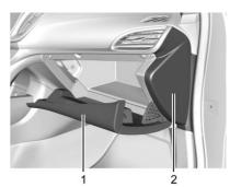
Open the glove box door (1) completely. Grasp the edges of the side instrument panel trim (2) and pull to remove from the instrument panel.
