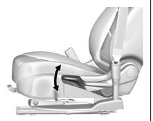
Move the lever up or down to raise or lower the seat.
