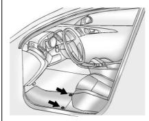
Reinstall by lining up the floor mat retainer openings over the carpet retainers and snap into position.
