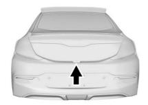
Press on the RKE transmitter to unlock all doors. Press the touch pad on the underside of the hatch and lift.
