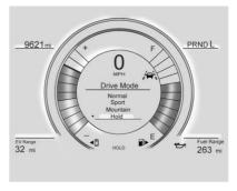
Use Hold Mode on a trip where it is expected that all of the electric charge will be depleted. Use Hold Mode mainly during highway or high speed driving to maximize both EV miles and fuel efficiency.
