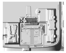
The rear compartment fuse block is in the center of the rear compartment under the load floor. Open the rear load floor door and remove the cover to access the fuse block.
