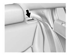
1. Pull the seatback release lever to unlock the seatback.
