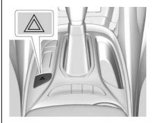
Press to make the front and rear turn signal lamps flash on and off. This warns others that you are having trouble.
