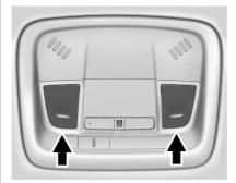
The front reading lamps are in the overhead console.
