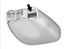
Separate the two halves of the transmitter using a flat tool inserted into the area near the key slot. Do not use the key slot.
