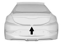
To open the hatch, press the touch pad on the underside of the hatch and lift after unlocking all doors. See  $Hatch \Rightarrow 42$ .
