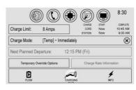
To cancel the temporary override to Immediate, touch the X next to the charge mode on the main charging screen.
