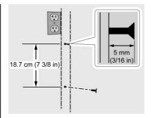
Mark and drill the mounting holes in a wall stud or suitable structure. Stay away from any power source.
