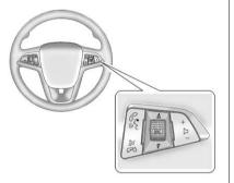
For vehicles with audio steering wheel controls, some audio controls can be adjusted at the steering wheel.
