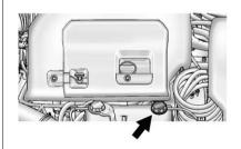
Check to see if coolant is visible in the power electronics and charger modules coolant reservoir. If coolant is visible but the coolant level is below the cold fill line, there could be a leak in the cooling system.
