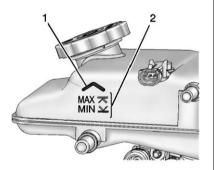
With the vehicle not running for at least one minute, the maximum fluid level (1) is at the top of the reservoir body. With the vehicle running, the fluid level should be in the proper operating range (2) between the MIN and MAX marks. If it is not, have the brake hydraulic system checked to see if there is a leak. After work is done on the brake hydraulic system, make sure the level, with the vehicle running, is in the proper operating range (2) between the MIN and MAX marks.
