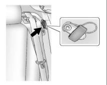
1. Remove the guide from its storage clip on the interior body trim next to the rear seat.
