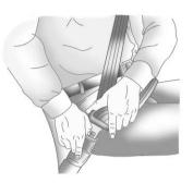
To unlatch the belt, push the button on the buckle. The belt should return to its stowed position.
