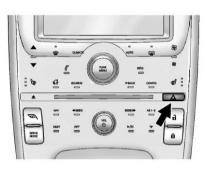
(Hazard Warning Flasher): Press this button to make the front and rear turn signal lamps flash on and off. This warns others that you are having trouble.
