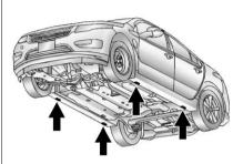
The front lifting points can be accessed from either side of the vehicle, behind the front tires.
