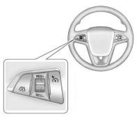
The cruise control buttons are on the steering wheel.
