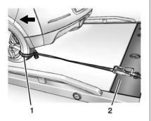
Secure the vehicle to the flatbed (2) using nonabrasive straps (1) through all four wheel openings and secure the straps to the flatbed (2).
