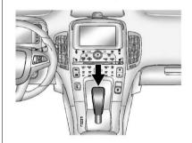
**P (Park):** This position locks the front wheels. It is the best position to use when starting the propulsion system because the vehicle cannot move easily.
