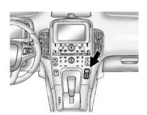
The vehicle has an Electric Parking Brake (EPB). The (P) switch is on the center stack. The EPB can always be activated, even if the vehicle is off. To prevent draining the 12-volt battery, avoid repeated cycles of the EPB system when the vehicle is off.
