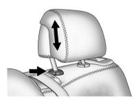
The height of the head restraint can be adjusted. Pull the head restraint up to raise it. Try to move the head restraint to make sure that it is locked in place. To lower the head restraint, press the button, located on the top of the seatback, and push the head restraint down. Try to move the head restraint after the button is released to make sure that it is locked in place.
