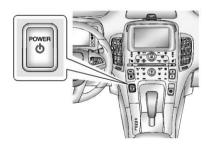
The vehicle has an electronic push-button start. The POWER button light flashes when the driver door is open and the vehicle is not on. The flashing light will eventually time out. The POWER  $\bigcirc$  button light is on steady when in ON/RUN power mode. When the vehicle is turned off, the POWER  $\bigcirc$  button light will turn off.
