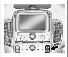
The power door lock switches are on the center stack.
