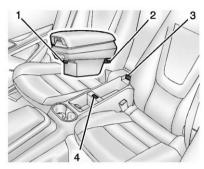
To install the armrest storage bin, align the bracket (2) on the rear of the armrest storage bin into the slot (3) on the rear console and push the armrest down until the latch (1) locks into the opening (4).
