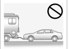
*Notice:* If the vehicle is towed with all four wheels on the ground, the drive unit could be
