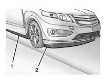
If the vehicle is parked off the shoulder of the road, at an angle that it cannot be pulled onto a flatbed, a hook/chain can be placed into either of the front torque box openings to pull the vehicle onto a flat surface. Make sure that the chains do not come in contact with the rocker panel (1) or the front fascia (2).
