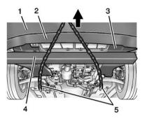
Place a 1.2 m (4 ft) X 102 mm (4 in) X 102 mm (4 in) wood beam (4) under the front cradle crossmember (3), and on top of both tow chains (5) to ensure the tow chains do not come into contact with the front fascia (1).
