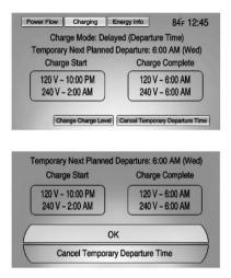
To cancel the temporary override of the Next Planned Departure Time, from the Temporary Charge Mode Status screen or pop-up, press Cancel Temporary Departure Time on the bottom of the touch screen.
