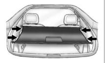
There is a cover for the rear cargo area. Use the four cargo cover loops to hook the cover to the side panels.
