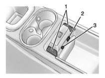
In the armrest storage area there is an auxiliary jack (2) and auxiliary power outlet (3). Cords from accessories can be routed through the pass-thru (1) on each side. See "Auxiliary Devices" in the infotainment manual.
