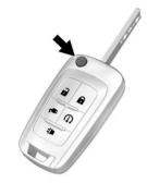
Press the key release button to extend the key. The key can be used for all locks.
