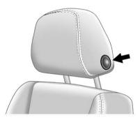
To raise or lower the head restraint, press the button located on the side of the head restraint and pull up or push the head restraint down and release the button.
