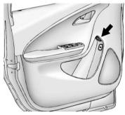
Press the fuel door button on the driver door for one second.
