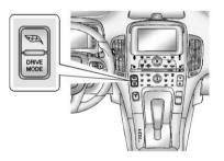
To view the Power Flow, Charging, and Energy Information, press the button on the center stack.
