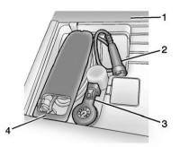
2. Open the rear hatch, lift the load support floor covering (1), and remove the charge cord (4). It is
