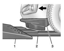
5. Ramps (2) are required for the front fascia (3) to clear the flatbed (1). The ramp height should be approximately 102 mm (4 in). Lower the flatbed onto the set of ramps.
