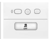
TCS can be turned off by pressing and releasing the TCS/ESC button on the overhead console. When TCS is turned off, (2) comes on, and the appropriate DIC message also displays. See *Ride Control System Messages on page 5-48*. With TCS turned off, the system does not limit wheel spin. Driving should be adjusted accordingly. See *Traction Off Light on page 5-22*.
