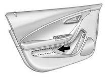
Slide an umbrella into the opening on either the driver or passenger door. Additional Storage Features
