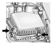
2. Remove the air cleaner cover. See Engine Air Cleaner/Filter on page 10-12.
