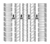
Treadwear indicators are one way to tell when it is time for new tires. Treadwear indicators appear when the tires have only 1.6 mm (1/16 in) or less of tread remaining. See *Tire Inspection on page 10-51* and *Tire Rotation on page 10-52*.
