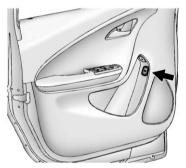
The charge port door release button is on the driver door inner trim panel. With the vehicle in P (Park), press the button for one second and release to open the charge port door. The charge port door can also be opened using the RKE transmitter. See *Remote Keyless Entry (RKE) System Operation on page 2-2.*
