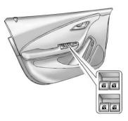
The window switches on the driver door control all windows in the vehicle. Each passenger door has a switch that controls only that window.
