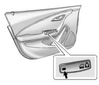
The rear window lockout switch is on the driver door. This feature prevents the rear passenger windows from operating, except from the driver position.
