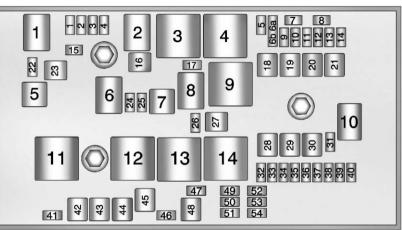
**Engine Compartment Fuse Block**
