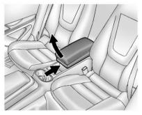
To remove the armrest storage bin, push the button and lift the armrest storage bin up.
