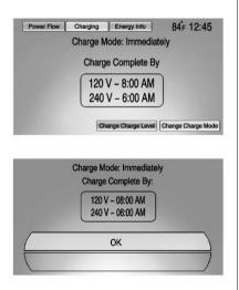
**Immediately:** The vehicle starts charging as soon as it is connected to an electrical outlet. See *Plug-In Charging on page 9-47*.
