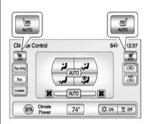
If available, the controls can be accessed while the vehicle is on by pressing the CLIMATE button on the center stack.
