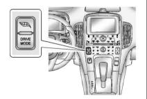
Press the DRIVE MODE button to display selectable drive modes in the Driver Information Center (DIC). Continue pressing to scroll through the modes.
