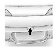
**Keyless Access:** To open the hatch with the vehicle locked, the RKE transmitter must be within 1 m (3 ft) of the trunk. Press the button on the underside of the hatch and lift up. See *Remote Keyless Entry (RKE) System Operation on page 2-2.*
