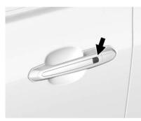
When the Remote Keyless Entry (RKE) transmitter is within 1 m (3 ft) of the driver door, the door can be locked and unlocked by pressing the door handle button. When unlocking from the driver door, the first press will unlock only that door; press again within five seconds to unlock all passenger doors. See *Remote Keyless Entry (RKE) System Operation on page 2-2.*
