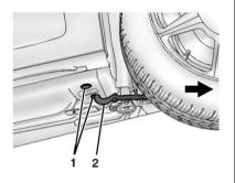
Place the tow chain hooks (2) into one of the torque box openings (1) behind the front wheels.
