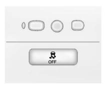
To turn off both StabiliTrak and TCS, press and hold the TCS/ ESC button on the overhead console, until (2) and 2 illuminate and the appropriate DIC message is displayed. See *Ride Control System Messages* on page 5-48. When StabiliTrak is turned off, the system will not assist with directional control of the vehicle or limit wheel spin. Driving should be adjusted accordingly. See *StabiliTrak*<sup>®</sup> OFF Light on page 5-23.
