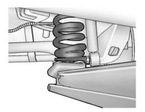
When lifting the vehicle from the rear, place the service jack directly under the spring seat.
