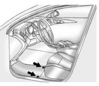
Reinstall by lining up the floor mat retainer openings over the carpet retainers and snap into position.
