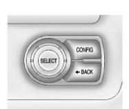
**CONFIG:** Press to select either the Simple or Enhanced instrument cluster configuration display.
