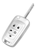
**(Unlock):** Press once to unlock the driver door. Press a second time within five seconds to unlock all doors.
