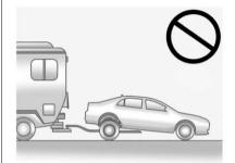
*Notice:* Towing the vehicle from the rear, with the front wheels on the ground, could damage the drive unit, and front fascia. Do not tow the vehicle from the rear with the front wheels on the ground.
