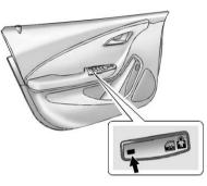
The rear door safety locks prevent passengers from opening the rear doors from inside the vehicle.
