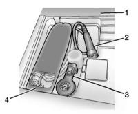
2. Open the rear hatch, lift the load support floor covering (1), and remove the charge cord (4). It is located near the tire sealant and compressor kit (3). Pull up on the charge cord handle (4) to release it from the handle clip.
