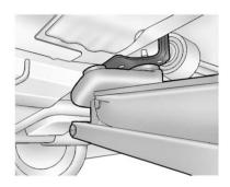
When lifting the vehicle from the front, place the service jack directly under the cradle mount. Ramps may be needed under the front tires to provide the necessary clearance for certain service jacks in this location.
