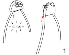
2. Attach the support tubes (I) to the frame. You should hear the click. Make sure, the parts are locked, pulling them back. Front support tube (I) should be bent inward, and the rear support tube is bent out. (As pictured)
