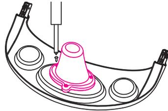
7. Attach the tray to the seat. You should hear the click. Make sure, the parts are locked, pulling them back.
