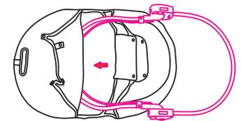
3. Thread the part D through the holes of case and fix both ends in plastic holes. You should hear the click. Make sure, the parts are locked, pulling them back.
