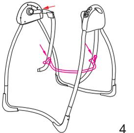
5. Install the seat on the frame. You should hear the click. Make sure, the parts are locked, pulling them back.
