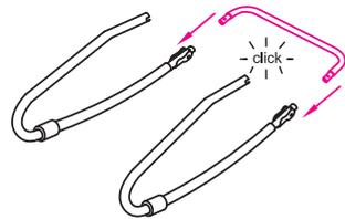
9. Install the seats on the rocking frame. You should hear the click. Make sure, the parts are locked, pulling them back.
