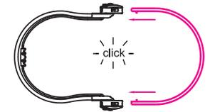
2. Put on the case (A) on the frame of seat (B and C).
