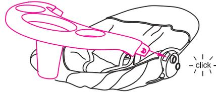
8. Connect the parts R and S. You should hear the click. Make sure, the parts are locked, pulling them back.
