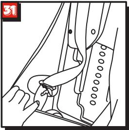
Insert the buckle tongues in the recess provided on the inside of the backrest. (fig.31)
