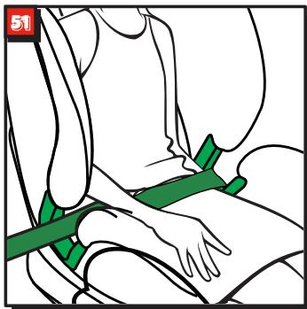
Place the lap belt section on the other side of the child seat in the lower belt guide. (fig.51)
