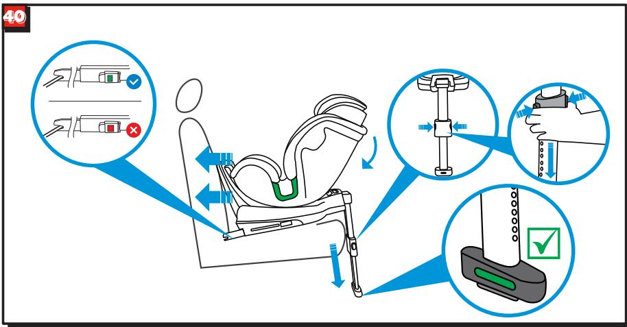
Install ISOFIX connectors (see section 4.7). Install support leg (see section 4.8). (fig. 40)
