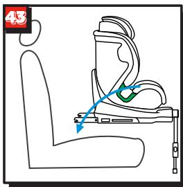
Pull away support leg from seat bottom, adjust anti-rebound bar at upright position. Rotate seat to forward facing (see section 4.5, fig.42). Place seat in the direction facing to the travel (fig.43). Install ISOFIX connectors (see section 4.7).
