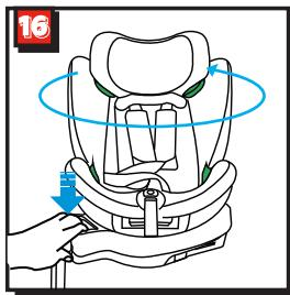
Pull rotation button at the same time rotate seat to intend direction. (fig.15,16)
