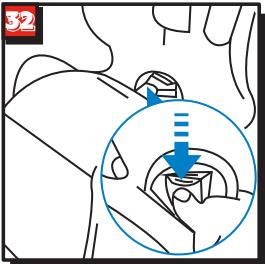
Open seat cover and fold the cover forwards, pull the harness buckle out of the cover. (fig.32)
