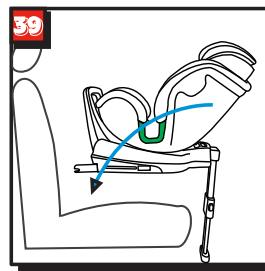
Pull away support leg from seat bottom. For more leg space adjust anti-rebound bar at incline position.
