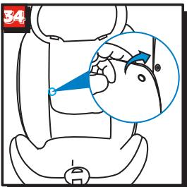
Close the two press studs and recovery seat cover. (fig.34)
