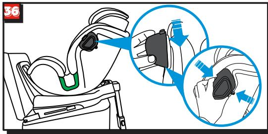
The side impact shield should install at the side which close to vehicle door.
