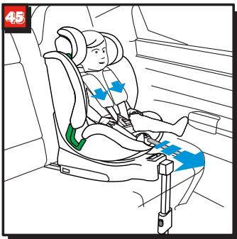
Have your child sit down in the child seat. Adjust headrest in proper height (see section 4.3), adjust harness and lock buckle (see section 4.1), and tighten harness, (see section 4.2) (fig.45)
