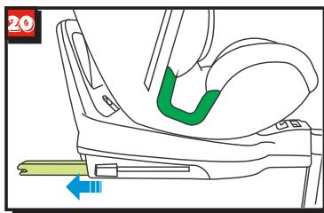
On both sides of the seat squeeze ISOFIX button and pull out ISOFIX connectors in longest position.(fig.19,20)
