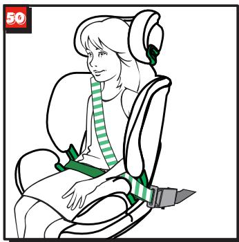
Place the diagonal seat belt section and lap belt section on the side of the vehicle seat belt buckle in the lower belt guide. (fig.50)
