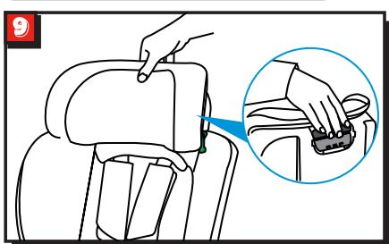
First loosen the harness. Squeezing headrest height adjuster at the same time slide headrest to shoulder height in accordance with the height of the child. (fig.9)
