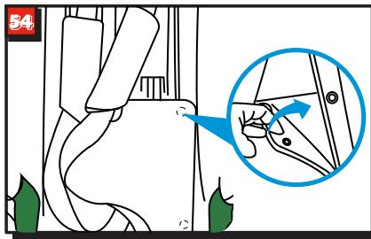
Loosen the press studs at the back of the headrest and remove the cover of headrest. Loosen the press studs and unzip at the back of seat cover. Pull forward and remove seat cover.
