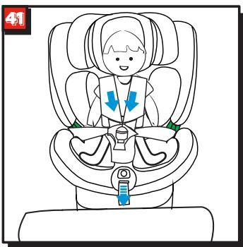
Have your child sit down in the child seat. Adjust headrest in proper height (see section 4.3), adjust harness and lock buckle (see section 4.1), and tighten harness (see section 4.2) (fig.41)
