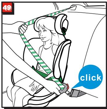
Have your child sit down in the child seat. Adjust headrest in proper height (see section 4.3). Pull out the vehicle seat belt and guide it in front of your child to the vehicle seat buckle. Engage the buckle tongue in the vehicle seat buckle. (fig.49)
