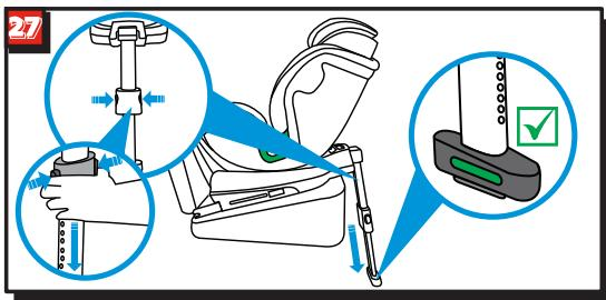
Pull the support leg away from the bottom of the seat until fully extended.
