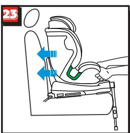
Slide the two ISOFIX connectors firmly into the insert guides until ISOFIX connectors engage with a clicking noise on both sides. ISOFIX button must turn green on both sides. (fig.21,22)
