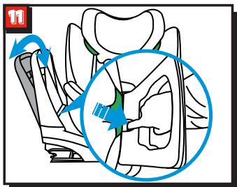
The anti-rebound bar has two positions reclined and upright. Forward facing only use upright position. Rotate child safety seat lateral facing. Pull up anti-rebound bar button then adjust the position of anti-rebound bar.
