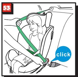
Have your child sit down in the child seat. Adjust headrest in proper height (see section 4.3). Pull out the vehicle seat belt and guide it in front of your child to the vehicle seat buckle. Engage the buckle tongue in the vehicle seat buckle. (fig.53)
