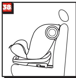
The side impact shield should install at the side which close to vehicle door.
