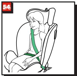
Place the diagonal seat belt section and lap belt section on the side of the vehicle seat belt buckle in the lower belt guide. (fig.54)
