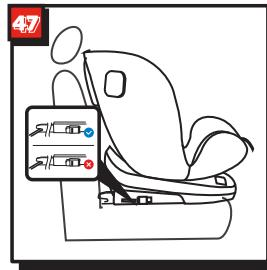
Rotate seat to forward facing (see section 4.5). Place seat in the direction facing to the travel. (fig.45,46)
