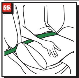
Place the lap belt section on the other side of the child seat in the lower belt guide. (fig.55)
