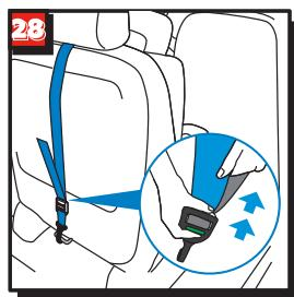
To tension the top tether, remove any slack by pulling on the free end of strap until it is suitably tightened. The top tether will be properly tightened when the tension indicator turns completely green. (fig.28)
