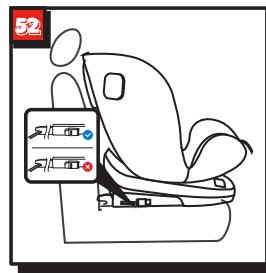
Rotate seat to forward facing (see section 4.5). Place seat in the direction facing to the travel. (fig.50,51)
