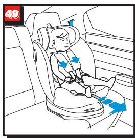
Have your child sit down in the child seat. Adjust headrest in proper height (see section 4.3), adjust harness and lock buckle (see section 4.1), and tighten harness (see section 4.2). (fig.49)
