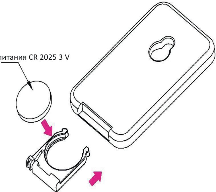
The diagram illustrates the battery compartment on the back of the device. A CR 2025 3V battery is shown being inserted into the compartment. Pink arrows indicate the direction of insertion and the location of the battery cover.
