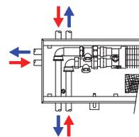
Electrothermal actuator can't be installed in the body of the trench heater due to limited internal space.
