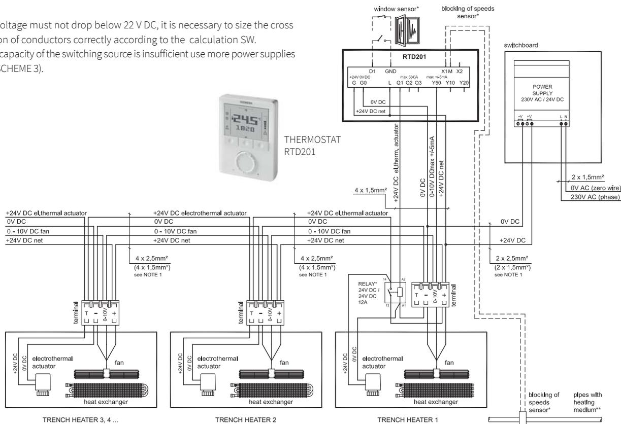
\*ccessories / \*\* The temperature sensor (block of revs) must be fixed on the tube, through which the heating medium freely flows and which is not closed by the actuator.
