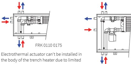
Electrothermal actuator can't be installed in the body of the trench heater due to limited internal space.
