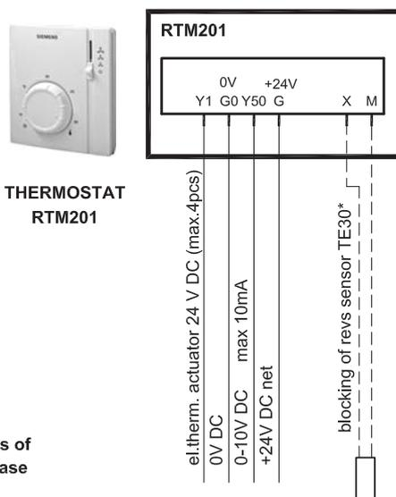
**Note:** Thermostat RTM201 can controll only 4 pcs of electrothermal actuator, for more pieces use please relay RL10, connection by Scheme 2
