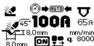
The power source automatically displays the width and depth of the groove that can be achieved with the current values (Pict. 4 Ref. G) at the relative processing speed (Pict. 4 Ref. E) set by the operator, and tells you which nozzle to use (Pict. 4 Ref. F) and the inclination in degrees that the torch needs to be maintained at during forward movement.
