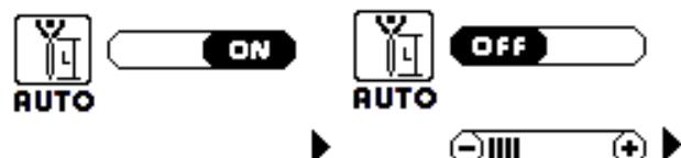
The factory default mode is AUTO ON which allows the power source to automatically and synergically adjust the length of the pilot arc based on the mounted torch, the installed consumables and the selected processing procedure. It is nevertheless possible to set this function on OFF so as to be able to manually adjust pilot arc length.
