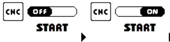
By setting this function on ON you enable START mode from the CNC relative to pins 3 and 4 of the AMP connector located on the rear of the power source and, at the same time, the manual start located on the machine's front adapter is disabled.
