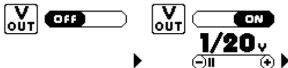
The factory default mode is OFF meaning that there is no voltage between outlet pins 5 (-) and 6 (+).
