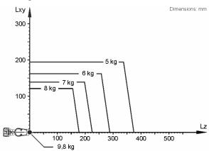
The KR 8 R2010-2 is designed for a rated payload of 8 kg in order to optimize the dynamic performance of the robot. With reduced load center distances, higher loads up to the maximum payload may be used. The specific load case must be verified using KUKA.Load. For further consultation, please contact KUKA Support.
