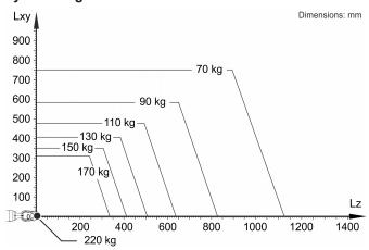
The KR 150 R3100-2 F is designed for a rated payload of 150 kg in order to optimize the dynamic performance of the robot. With reduced load center distances, higher loads up to the maximum payload may be used. The specific load case must be verified using KUKA.Load. For further consultation, please contact KUKA Support.
