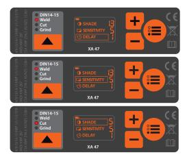
() You can adjust the function values for the WELD mode and DIN14-15 mode only. For the CUT and GRIND modes, the values of sensitivity and delay remain the same as they were in WELD mode, and the shade value changes to 4 for GRIND and to 5 for CUT.
