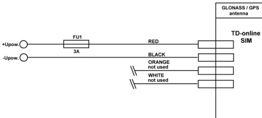
**APPENDIX 3.** Sensor connection diagram in normal operation mode with auxiliary sensor TD-500
