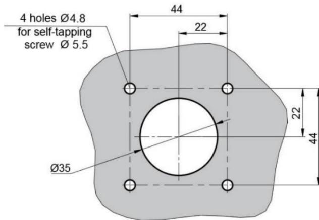
**APPENDIX 5. Sensor installation on the tank**
