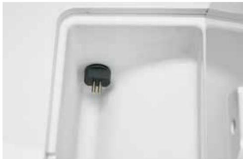
The quality of the distilled water being used is guaranteed by the **conductivity sensor incorporated in the tank** and an efficient warning message/alarm system. If the water is of unsuitable quality, the sterilizer informs the user with appropriate messages and prevents the use to avoid damage risks.
