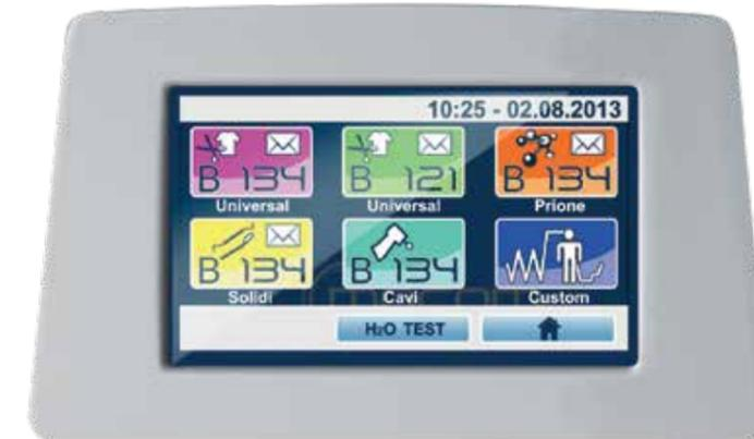
Sterilization cycles can be selected quickly and directly via the programme-associated icons on the touch-screen. The display also allows the user to select the language, manage users and personalise the sterilizer exactly as desired.
